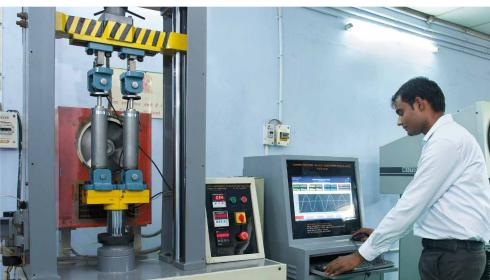
Advanced testing rigs and specially designed test procedures help in improving product design and error proofing of manufacturing processes. This ensures that shock absorber performance, reliability and life span benchmarks are fully achieved.
